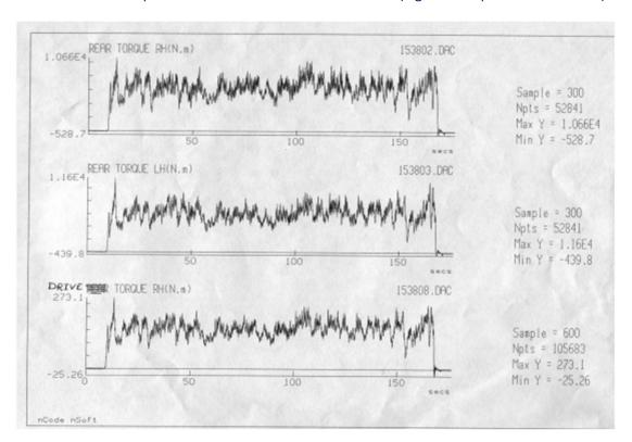
This is a commonly use solution for vehicle testing purposes and in order to determine the power on drive shaft, a speed measurement associated to torque will directly solve the problem.
