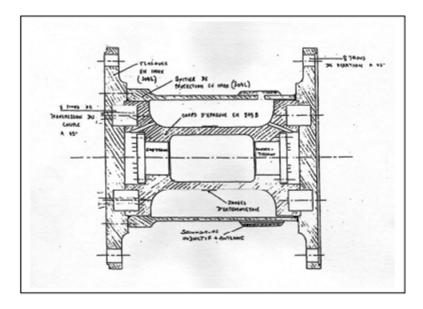
The picture shows an instrumented shaft. Both flanges, left and right are attached to sensitive mechanical part by means of screwed cylinders, this ensure stiffness integrity of the proof body and
