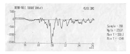
Transient torque measurements are transmitted so one can see what is happening to the torque when the wheel shocks a rock or a side walk.
