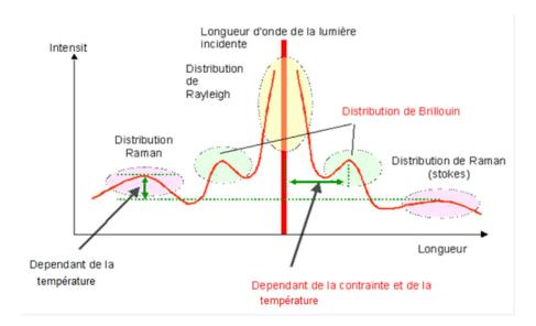
The light pulse is travelling all along the fiber scattering, at each point where a phenomenon occurs, will cause the frequency and amplitude drift that will be measured.
