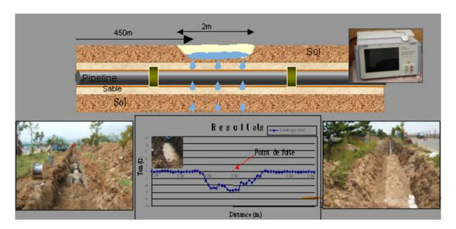
If, rare cases, fluid temperature and environment are suspected to be at exact same value, the trick will be to heat the fiber optic so a difference can be seen. Fiber optic line is then coated, under outside coating with an electrical conducting material. This coating will we powered with a generator and raise fiber optic cable to a determined temperature.
