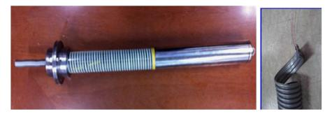
Then the fiber optic will be used as piezometer. Coupled to an inclinometer length, this assembly can fit dykes and inform on the movement inside the structure in same time than on water flow. This will lead to possible detections and locations of water flow in the structure and makes possible internal erosion detection and location.
