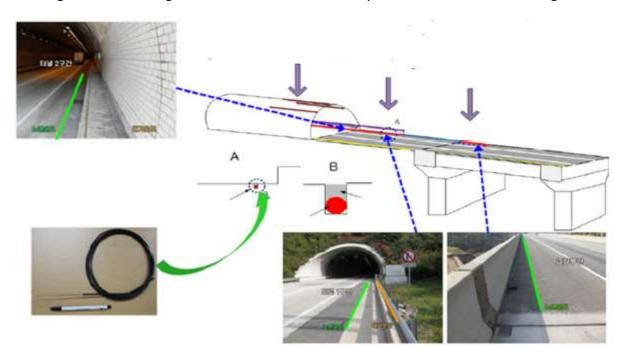
At the other end fiber optics will sense increases in temperature and warn quickly on burning start. Fire detection and location may be added simply to a fiber optic instrumentation.
