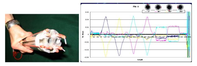
This makes available inclinometers all along the inside of a drilling as long as it is tightly maintain in the hole. Kilometers of inclinometers chain can therefore be achieve either in a drilling or along of a tunnel.
