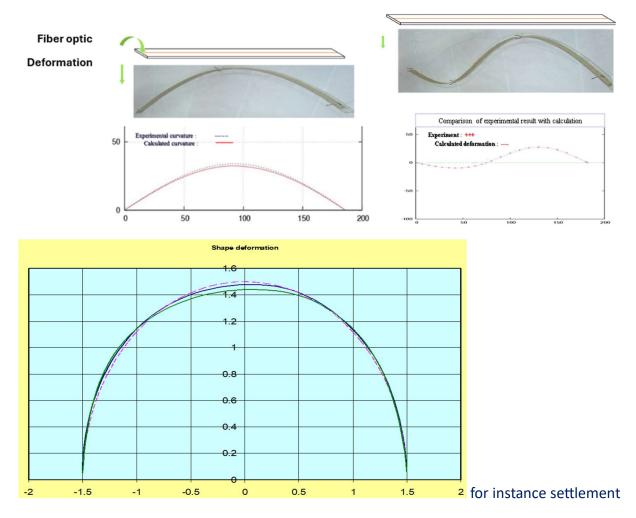
When it comes to determine the sense of application of the load, the fiber optics may be assembled as an inclinometer.
